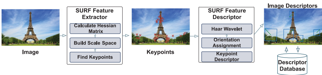
Fig. 5. Image matching pipeline.
